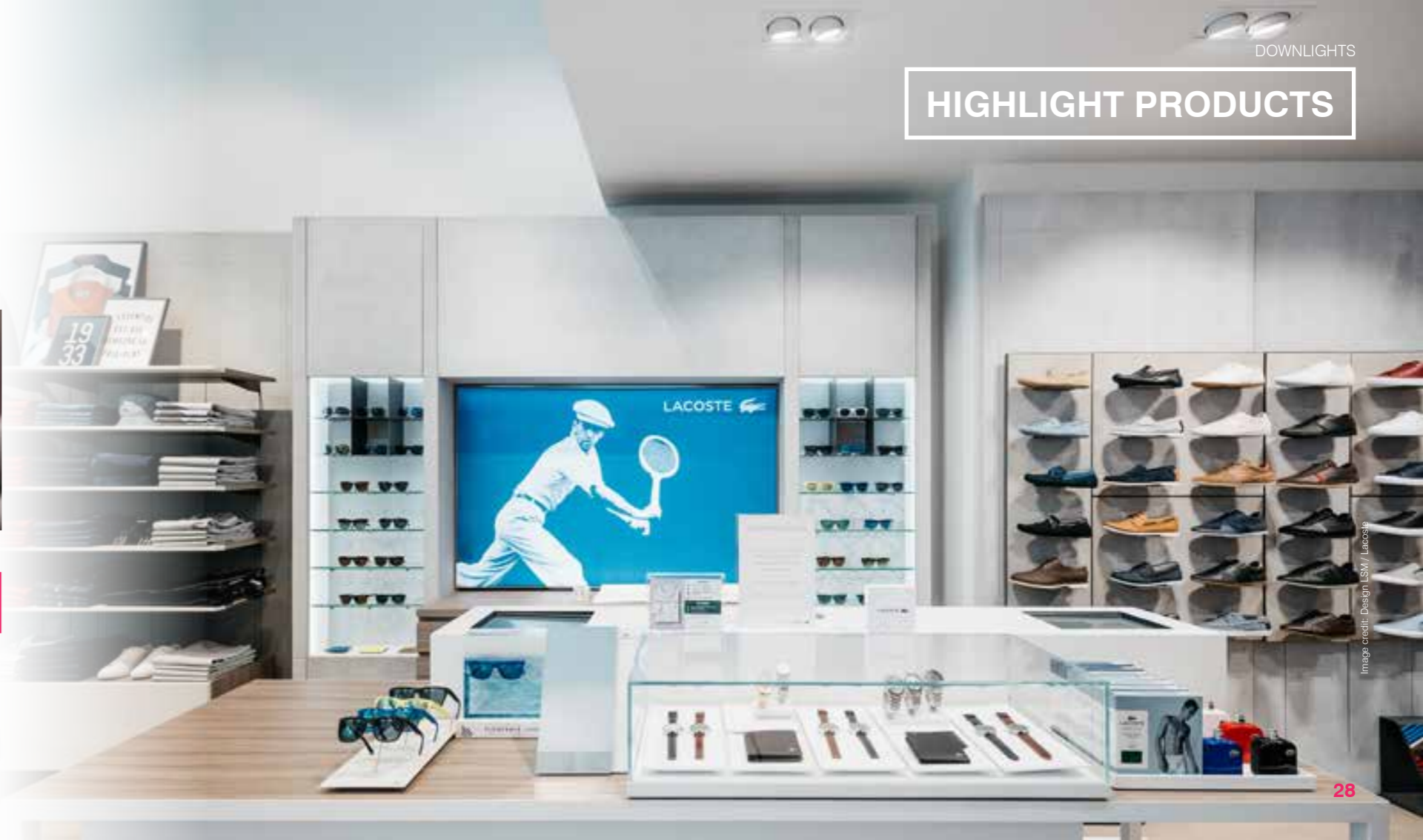
VISION | Recessed adjustable downlights with 4000K Xicato LED. Shown here in double or triple lamp versions, with a matt white trim and backplate.
