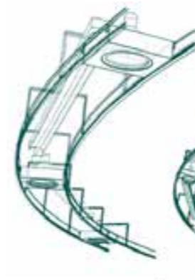
Price Waterhouse Coopers | KENO Curved Made-to-Measure lighting frame system with integrated downlights and illuminated linear sections.
