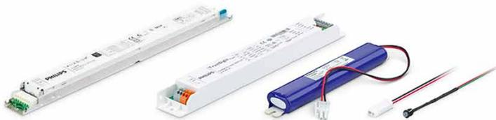
The integrated Emergency conversion (Standard/DALI) will run the driver at 30% output for 3-hours. The converted drivers output is shared equally across each connected board, illuminating the entire length in emergency mode. This improves uniformity to comply with emergency regulations.
